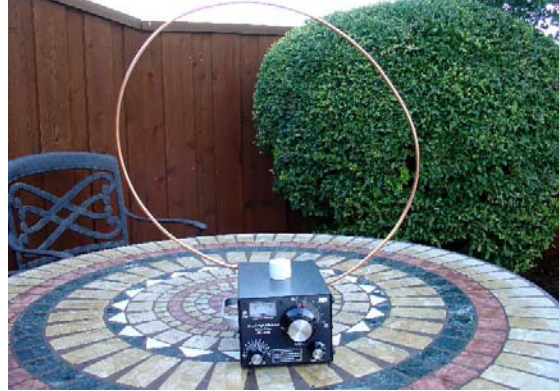
5-ft 17-10m copper loop and MFJ-935B
