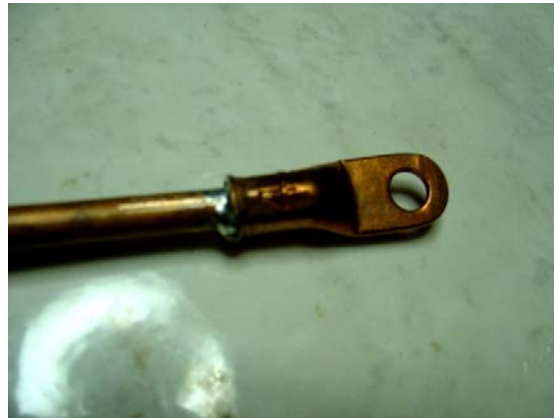
Tubing & lug after crimping & soldering
