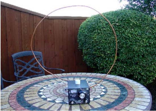
6-ft 20-15m copper loop and MFJ-935B
