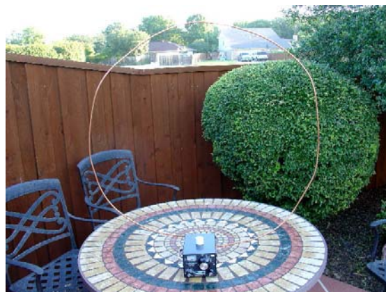
10-ft 30-20m copper loop & MFJ-935B
