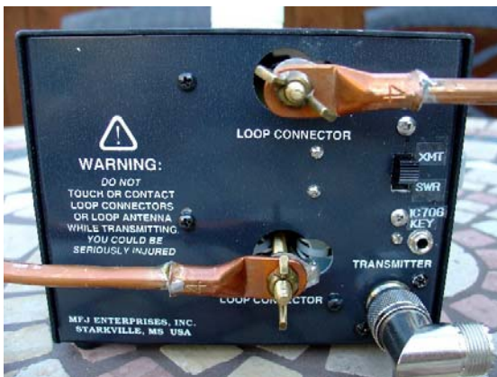
MFJ-935B copper loop mounting
